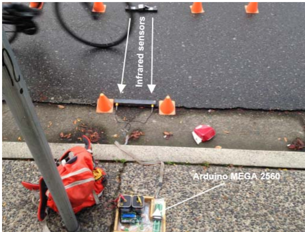
FIGURE 2. Custom-made bicycle speed measurement system, here shown in action during data collection
